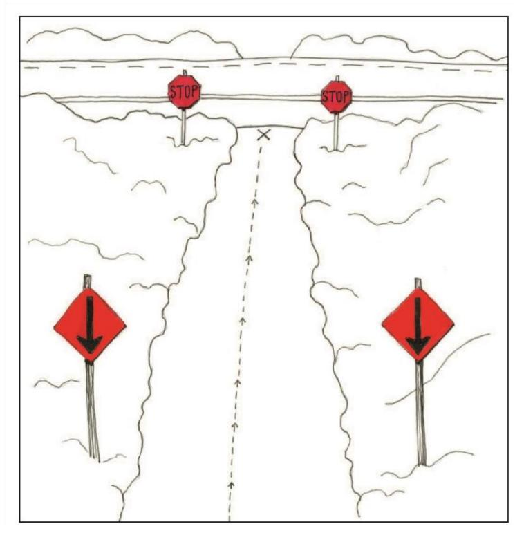
Typical road crossing, no roll or slide through — must stop.
